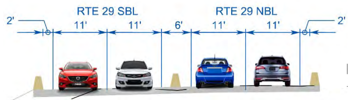
Figure 13: Barrier Separation of Bi-Directional Traffic
